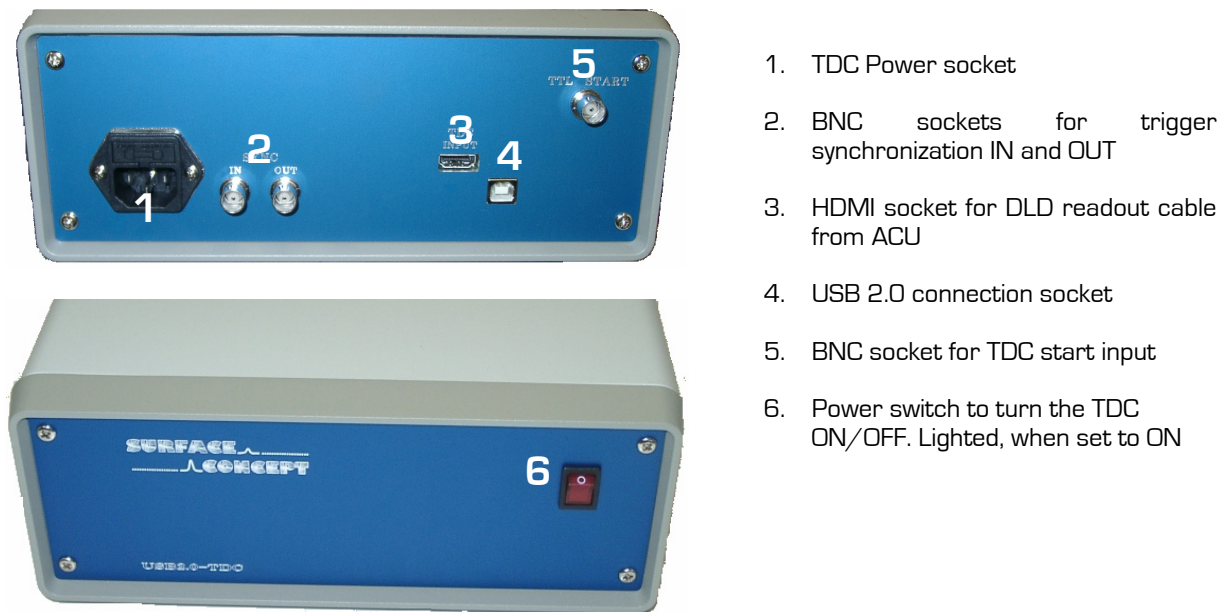
Figure 11: Layout of the Double USB2.0-TDC
