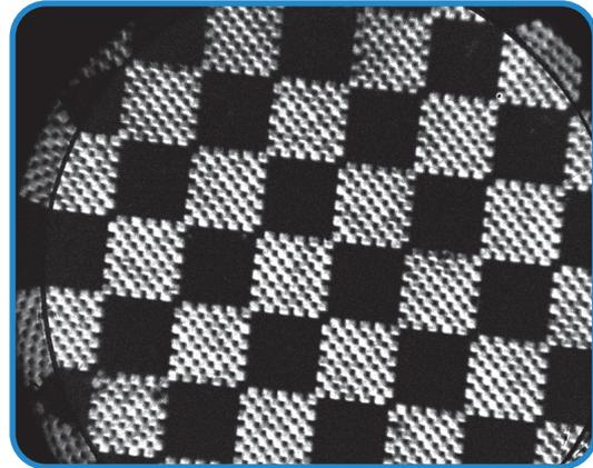
Phosphor screen detector image of a chessy sample taken with a ReconFlex 800 in normal camera mode (left) and same image using the blob finder mechanism at 1577fps (right). The blob finder returns true count rates and suppresses any background or stray light very efficiently."
