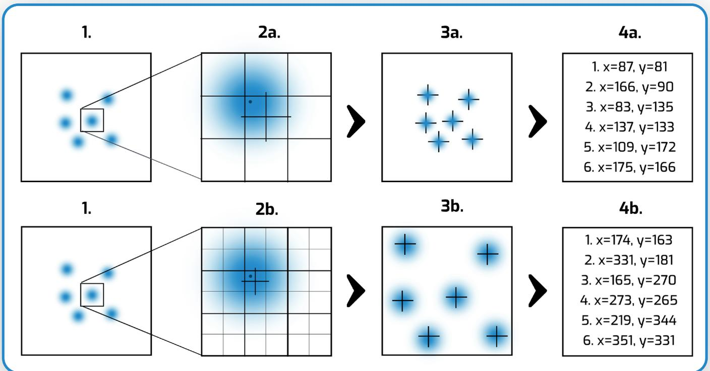
The blob finder mechanism enables precise and fast finding of peak coordinates and their counting. It recognises single peak intensities and their coordinates (no. 1, 2a and 3a) directly on the hardware and provides a coordinate list (4a) on the fly. Coordinate lists can be streamed directly assigned to frame time stamps and ADC values. The software assembles virtually noise free images from the coordinates.
