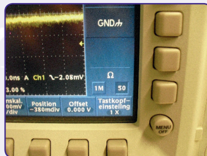
Figure 6: 50Ohm termination setting of oscilloscope input channel.
